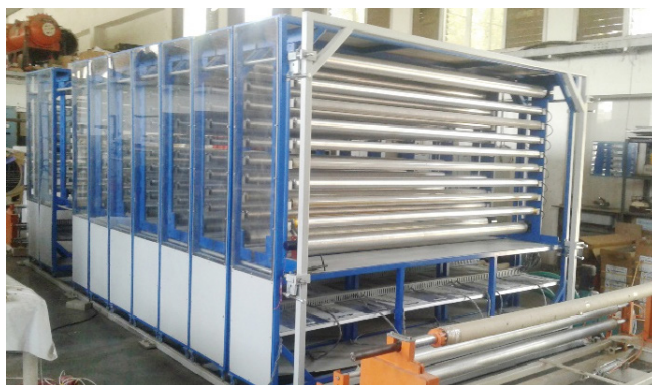
Figure A.3.8 Inline plasma treatment system for textile
