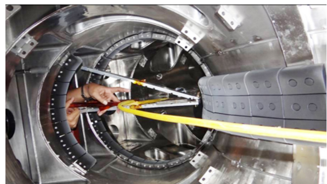
Figure A.1.2.2 Setup for Magnetic diagnostics coils in-situ calibration
