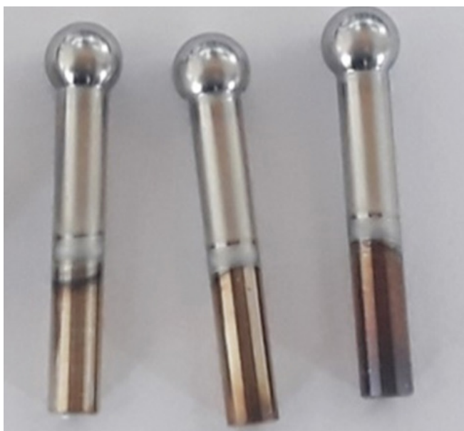
Figure A.3.4 Plasma Nitrided 17-4 PH samples for Tribology studies
