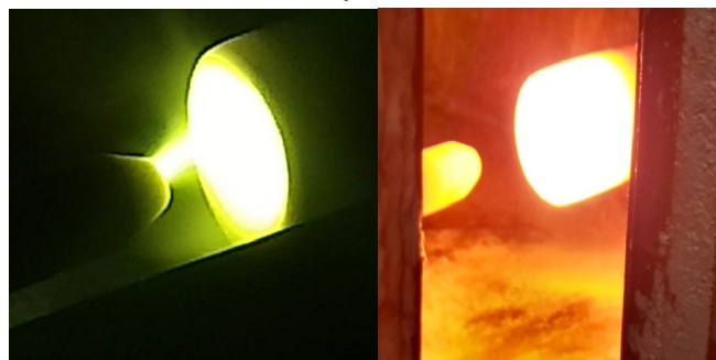
Figure A.3.6 (a) Plasma torch during operation viewed through UV screen (b) Red hot graphite electrodes immediately after operation
