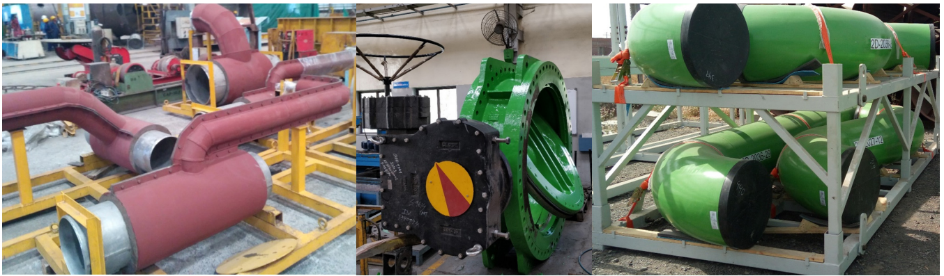
Figure B.2 Parts of water cooling system (a) Pipe Spools (b) valve and (c) Pipe spools
