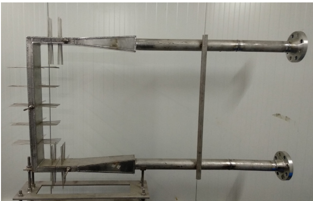
Figure 2.4.2 Test section for studying magneto-hydrodynamic (MHD) effect for Pb-Li flow
